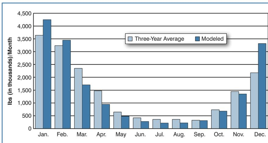
Figure 2: Steam calibrated model and metered use.
