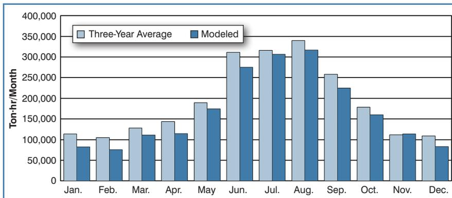
Figure 3: Chilled water calibrated model and metered use.
