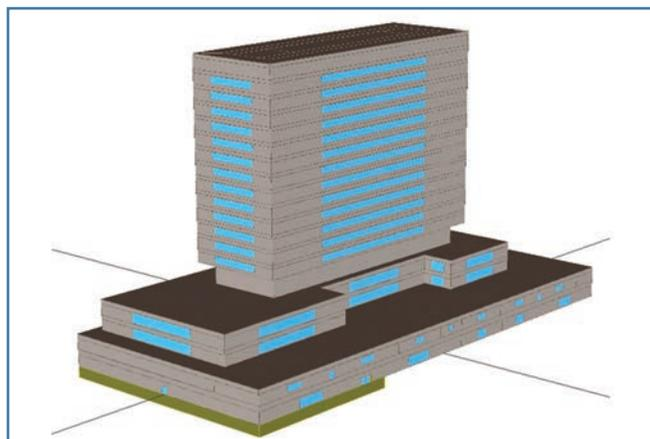
Figure 1: Sketch of energy model geometry.
