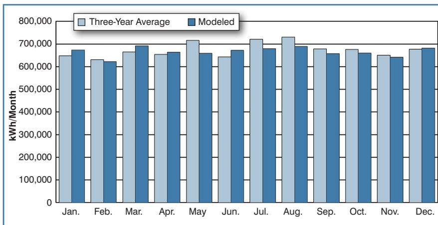
Figure 4: Electricity calibrated model and metered use.
